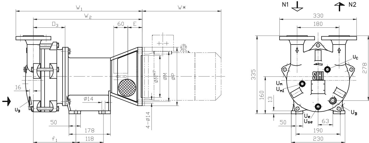
N 1 = Gas inlet DN 40 吸气口 DN40
